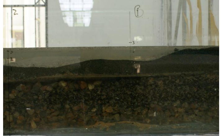
Fig. 4.a U/S sediment profile after Flushing Grid No.1 and 2
